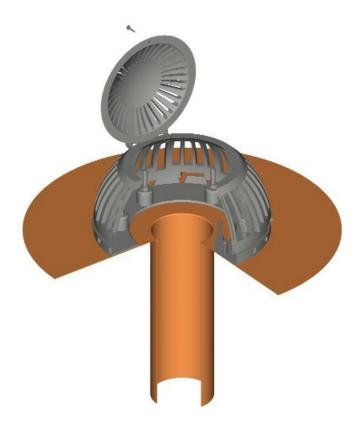
Notice to plumbing / roofing contractor: When a copper drain sleeve must be cut for adjustment to appropriate length, avoid the use of vibrating tools that could generate fissures in the copper flange or sleeve along the solder. Rather utilize a circular cutter.
