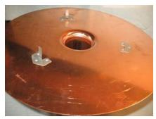
each membrane ply. Once all membrane plies in place, the dome strainer shall be positioned and finally anchored in place by the 3 anchor strips to be folded onto the strainer base ring through their respective openings. When placing his Ultra Dome drain order, the roofer shall specify whether or not the dome strainer has to be already shop-anchored to the drain flange.
